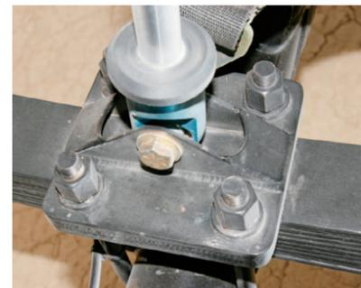
▲ Reinforced factory spring plates were initially part of the build, but they bent while the U-bolts were being torqued. S.I. obliterated the problem by making new spring plates out of (you guessed it) chromoly plate. Two pieces of 3/8-inch plate were cut out and welded together to form the base. "Bomb-proof" comes to mind.
