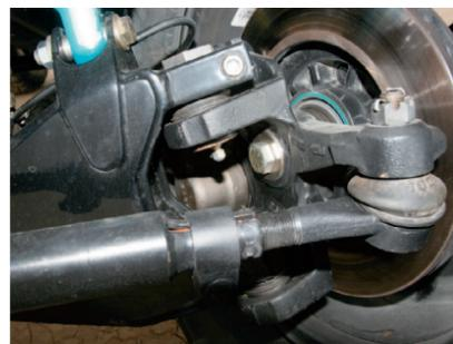
▲ Stock 2WD Ranger spindle snouts have a habit of pulling out of the steering knuckles that they're attached to. The team at S.I. didn't merely fix this problem, they smashed it. In place of the stock spindle, they pressed a custom 4WD-style spindle into place, and then welded it to the knuckle. As if pressing and welding weren't enough, the bolt you see on the back side of the knuckle goes through and adds a third layer of spindle retention.
