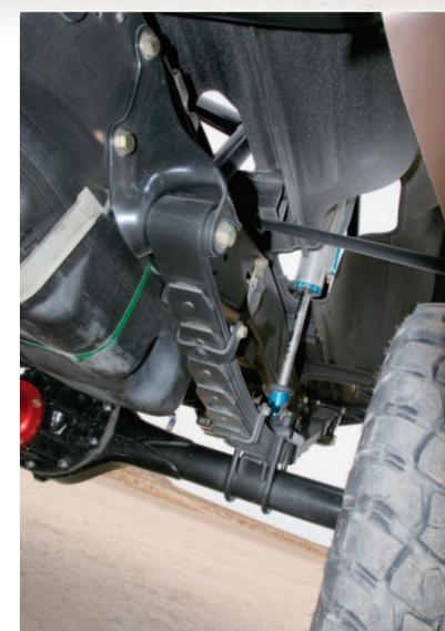
▲ Deaver leaf packs are part of the S.I. ranger formula. The spring-over configuration was retained, but the rear shackles were flipped to reduce the springs' negative arch at full bump. The factory spring hangers were retained, but the rivets were drilled out and replaced with grade-8 fasteners.
