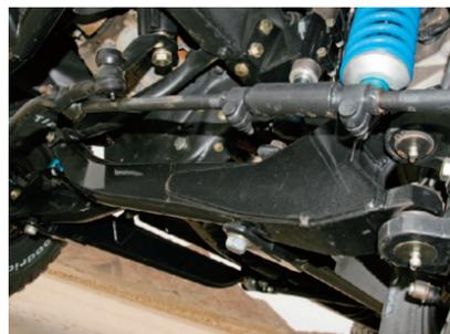
▲ Like the engine cage, the S.I. I-beam front end combines chromoly tubing and plate, melded using a TIG machine. These 4-inch wider-per-side I-beams pivot from the original brackets, so they're the un-equal length factory configuration. The steering adjusters were lengthened using 1.25-inch solid stock which was externally sleeved with 1.5-inch chromoly tubing.
