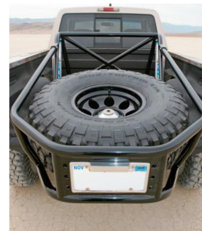
▲ This is one spare tire carrier you won't want to nerf. The spare is held down by a nut that uses a special internal spline configuration for extra security.
