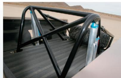
▲ The bed cage is made from 1.75-inch, 0.120-wall chromoly tubing, and provides a home to a pair of 16-inch-stroke King bypass shocks. The interior of the bed was coated with Line-X to deaden sound and preserve longevity.
