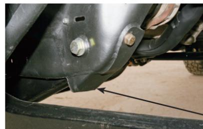
▲ Tom re-welded the factory seams on the I-beam crossmember. He also added reinforcing washers to the beam pivot points. A small pocket was added to the bottom of the crossmember (arrow) to facilitate additional droop travel. There are 20 inches of front suspension travel on tap.
