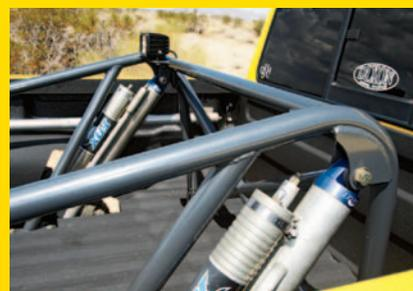
▲ A pair of Fox bypass shocks controls 16 inches of rear wheel travel.
