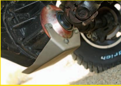
▲ The stock rearend was ditched for a custom Currie 9-inch stuffed with 4.88 gears and a spool for trouble-free (albeit not that pavement friendly) traction. The skid plate is another meticulous S.I. Motorsports creation.
