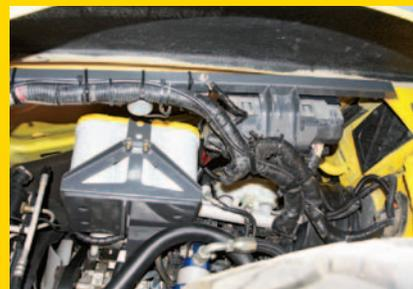
▲ Did we mention attention to detail? Take a look at the custom S.I.-built battery tray and the equally slick fuse box bracket. This stuff takes extra time during a build, but it makes the resulting truck infinitely more reliable as well as easier to work on.
