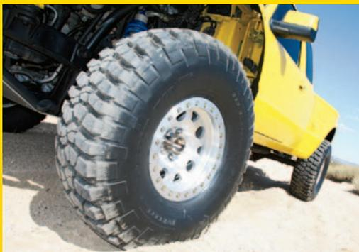
◀ Here's a wheel and tire combo we've seen before: KMC Enduro Beadlocks wrapped with BFGoodrich KM2 Mud-Terrain tires. This is a strong combination that affords traction over a variety of surfaces: perfect for a triple-duty truck. Fifteen-inch wheels clear the stock Ranger brakes and afford the tallest, most forgiving tire sidewall possible.
