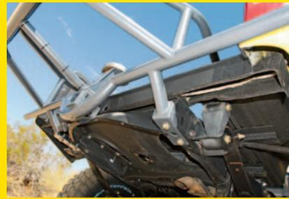
▲ The rear bedcase-and-bumper combo is a joint effort by Dixon Bros. Racing and S.I. Motorsports. The main structure is by Dixon, and S. I. added custom touches in the form of the hitch receiver and the tire carrier.
