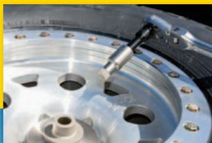
▲ Custom security splines keep the spare in place until it's needed.
