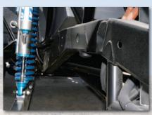
▲ To buy additional bumptravel, Tom kicked the rear framerails 6 inches upward. The frame has been boxed and gusseted in critical areas. The rear suspension cycles through 28 inches of travel: 14 inches up and 14 inches down. King shocks are used at every corner.
