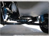
Tom tied the tranny crossmember into the radius-arm pivot brackets, then connected it to the suspension/engine crossmember. This structural bracing is hidden by a custom aluminum skidplate, which keeps the 400 small-block and the TH400 from getting smacked by errant rocks.
