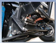
▲ In front of the kingpin equal-length I-beams is an S.I. swingset steering system. This system is designed to precisely follow the suspension movement for zero bumpsteer throughout the front end's travel. The one-off Chevy kit cycles at 22 inches total: 12 inches of bumptravel and 10 inches of droop travel. Tommy Lee built the steering box, custom pump, and ram assist.
