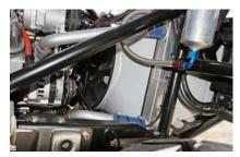
▲ Big ponies put out big heat, so a Ron Davis aluminum radiator sits up front to supply the chill. Tom's TIG-welding expertise also includes aluminum: He built the radiator shroud and sectioned the aluminum radiator tubing.
