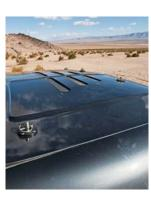
needed to get rid of the heat; ditching the fenderwells helps too. SI Motorsports took the concept a step farther and integrated six screened vents into the Autofab hood that's held in place with another sextet of Autofab hood pins.
