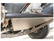
▲ As previously stated, this truck was designed to be easy to work on. If the Ken Mogi-built C6 needs to be dropped for maintenance, the entire framework and skidplate beneath it can easily be unbolted for access. A pair of MagnaFlow mufflers quiets down things while preserving the throaty note produced by the 650 ponies under the hood. The mufflers bolt to custom SI headers.
