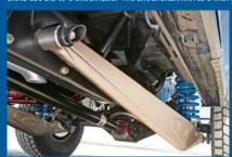
shocks require lots of damping to control the wheels. The higher damping rates mean lots of heat gets generated, which in turn means the shocks run hot. Hot shocks will fade if they get hot enough. I designed this four-link to use a 1.2-to-1 ratio. The shocks move faster than they would at a 2-to-1 ratio, but less damping is required, so the shocks run cooler."
