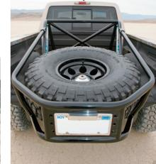
▲ This is one spare tire carrier you won't want to nerf. The spare is held down by a nut that uses a special internal spline configuration for extra security.
