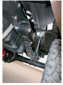
▲ Deaver leaf packs are part of the S.I. ranger formula. The spring-over configuration was retained, but the rear shackles were flipped to reduce the springs' negative arch at full bump. The factory spring hangers were retained, but the rivets were drilled out and replaced with grade-8 fasteners.
