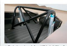
▲ The bed cage is made from 1.75-inch, 0.120-wall chromoly tubing, and provides a home to a pair of 16-inch-stroke King bypass shocks. The interior of preserve longevity.
