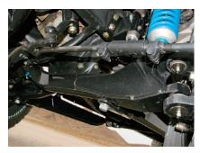
▲ Like the engine cage, the S.I. I-beam front end combines chromoly tubing and plate, melded using a TIG machine. These 4-inch wider-per-side I-beams pivot from the original brackets, so they're the un-equal length factory configuration. The steering adjusters were lengthened using 1.25-inch solid stock which was externally sleeved with 1.5-inch chromoly tubing.
