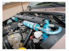
▲ S.I. Motorsports built Tim's engine cage from 1.5-inch, 0.120-wall 4130 chromoly tubing and 1/8-inch-thick chromoly plate. TIG welding was used exclusively on this build. The engine cage bolts to the frame using grade-8 hardware. Fourteen-inchstroke King coilovers help provide 20 inches of front wheel travel.
