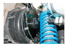
▲ Getting the coilovers to mount at the correct angle was no easy task. The HVAC blower motor was in the way. Rather than push the coilover forward to an angle that wasn't ideal, Tom built an adapter plate for a shorter blower motor. On the driver's side, a new master cylinder with exit ports on the passenger's side was used to keep the brake lines away from the coilover.
