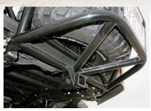
▲ The underside of the spare tire carrier is no less impressive. S.I. integrated a hitch just in case Tim wants to do some towing.
