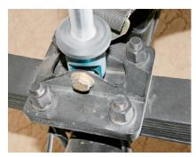
▲ Reinforced factory spring plates were initially part of the build, but they bent while the U-bolts were being torqued. S.I. obliterated the problem by making new spring plates out of (you guessed it) chromoly plate. Two pieces of 3/8-inch plate were cut out and welded together to form the base. "Bombproof" comes to mind.
