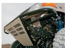
▲ A bolt-on S.I. front bumper leads the way. The screened vent holes keep large chunks out of the radiator
